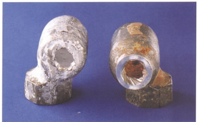
Alloy steel nozzles after about 300 operating hours
