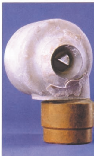
A silicon carbide nozzle after about 25.000 operating hours
